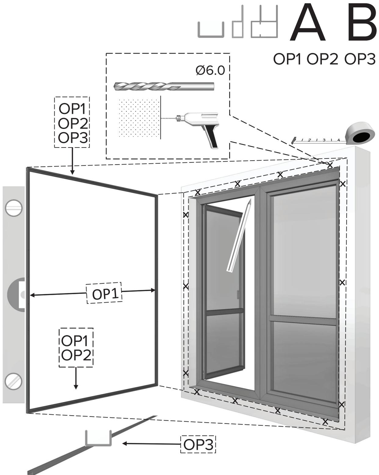
Once the slides have been prepared, try them on at the intended installation location and mark the limit points at which they are to be located, making it easier to move the required dimensions.
